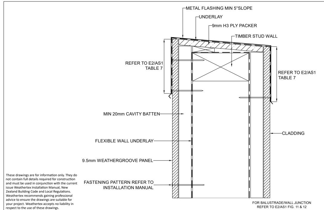
Weathertex | Drawing Name: | CAVITY FIX INSTALLATION - PARAPET (WEATHERGROOVE RANGE) | NTS | A.MOATE | R.STUART | 07.09.22 | NZ-WG-CF-19 | A4
